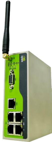
InRouter6x5 series products are M2M wireless routers that integrate 3G network and virtual private network (VPN) technologies. The products meet fundamental needs of field communication in industry, support international commercial UMTS (HSPA+), CDMA2000 1x EV-DO (Rev. A), TD-SCDMA networks, and respectively backward compatible with EDGE, CDMA 1X and GPRS network.
