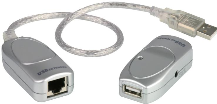
UCE60 lets you locate your USB device or hub up to 60m (198 ft) from your computer, overcoming the typical USB cable limitation. It conditions the USB signals to communicate up to 60m using low-cost Cat 5/Cat 5e/Cat 6 cable.
