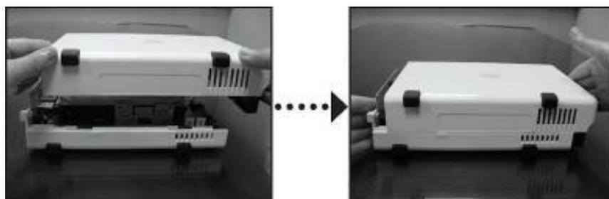
7. Fix the case with the 2 case screws provided.
