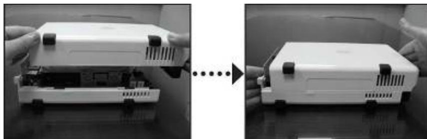
9. Fix the case with the 2 case screws provided.
