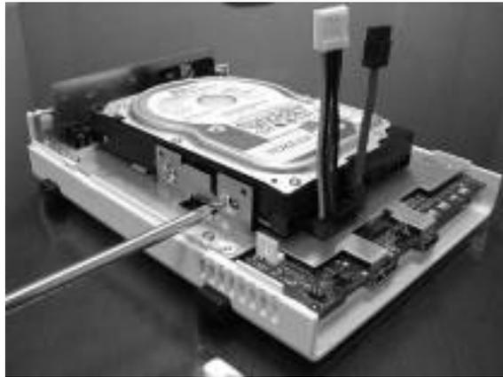
7. Connect the HDD Data Cable and HDD Power Cable to the motherboard. (Skip this step if the Disk Station is a cable-less model.)
