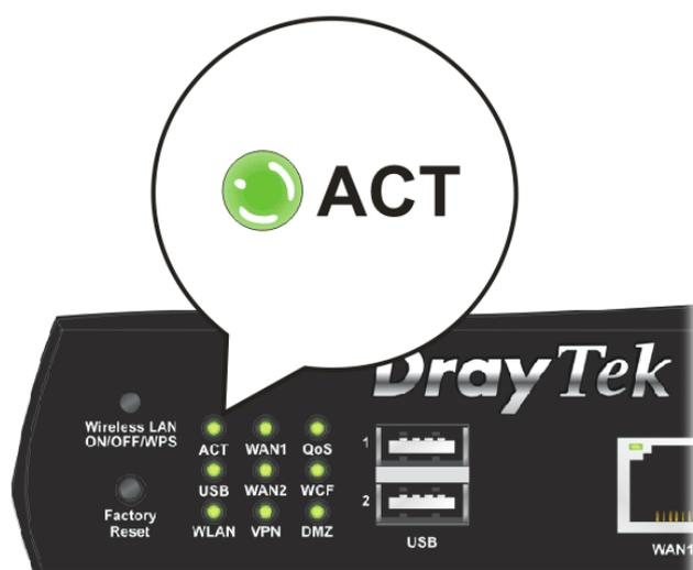
3. If not, it means that there is something wrong with the hardware status. Simply back to “**2.1 Hardware Installation**” to execute the hardware installation again. And then, try again.
