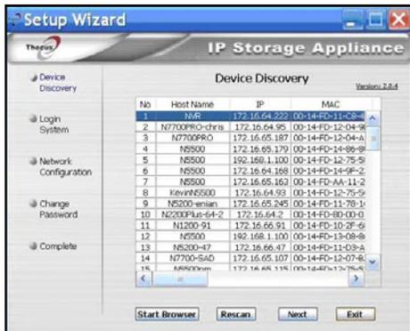
To change the IP address, simply click the desired system from the discovery list and follow the wizard step-by-step to complete the settings.
