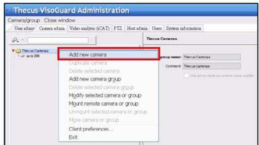
For each newly added camera, enter the proper camera settings and confirm them using the Save button. The camera will appear under the Camera group.
