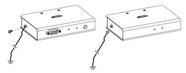
2. Make sure that the computer that the CE250AL connects to and the monitor that the CE250AR connects to are properly grounded.
