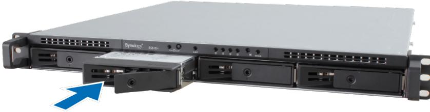
**Note:** Make sure the tray is pushed in all the way. Otherwise, the drive might not be able to function properly.
