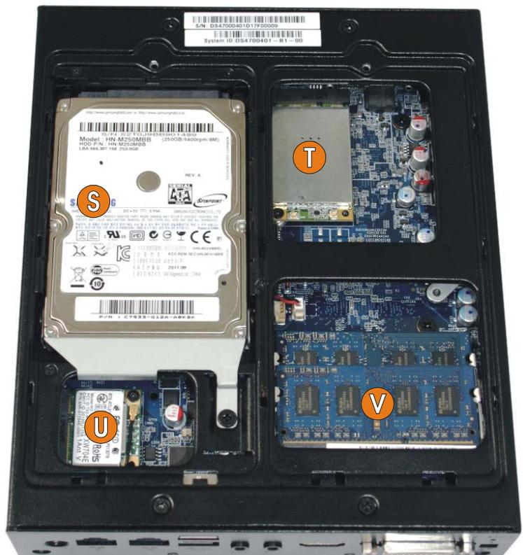
\*) The WLAN module is included in the scope of delivery in the form of a Mini-PCIe card. The other components such as hard disk, SSD, memory modules, other Mini-PCIe cards or mSATA modules are not.
