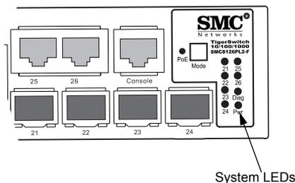
**Figure 1-4 System LEDs**
