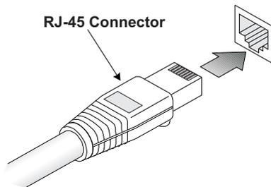
Figure 3-1 RJ-45 Connections
