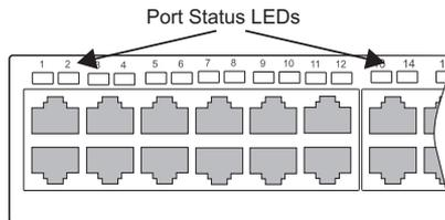
Figure 1-3 Port LEDs
