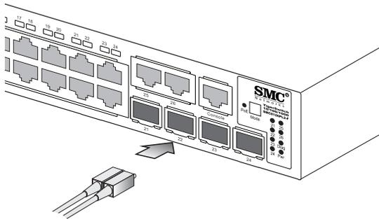
**Figure 4-3 Making Connections to SFP Transceivers**
