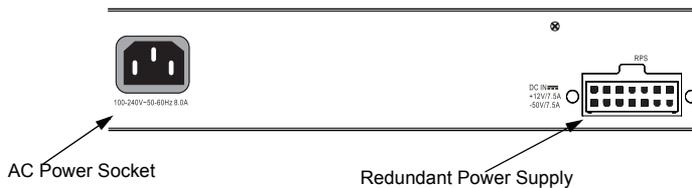
Figure 1-6 Power Supply Socket
