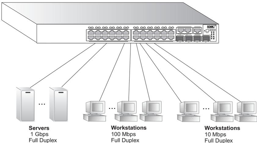
**Figure 2-1** Collapsed Backbone
