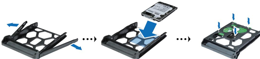
4 Insert the loaded drive tray into the empty drive bay. Make sure the side marked with "UP" is facing up, and insert the drive tray into the empty drive bay. You should hear a click when the tray is locked in place.
