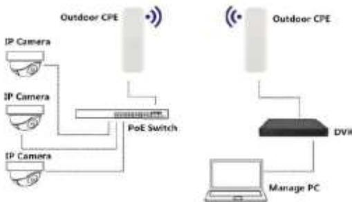
4.PTMP Working Diagram of Outdoor CPE work with Multiple IP Camera
