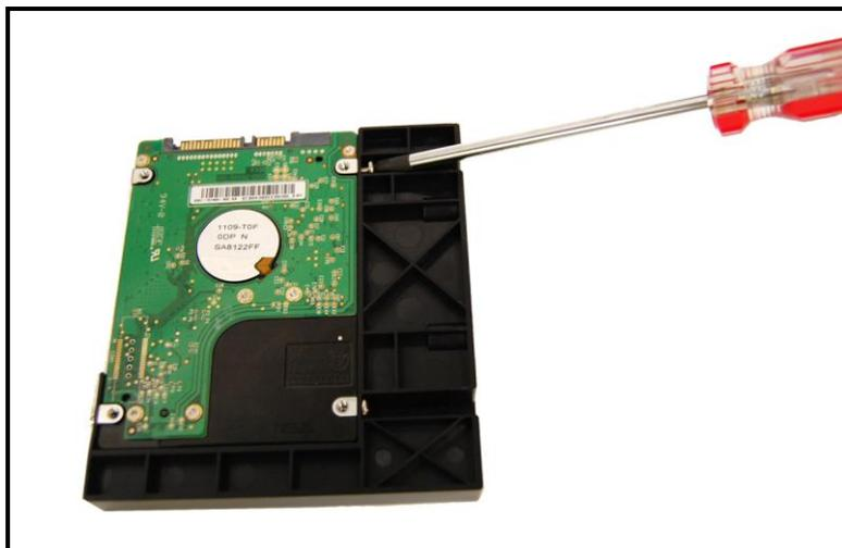
Slide the 2.5” Disk Holder into the hard disk bay and push it all the way back until it is connected to the SATA connector. Secure the Disk Holder with the 2 hard disk screws provided.
