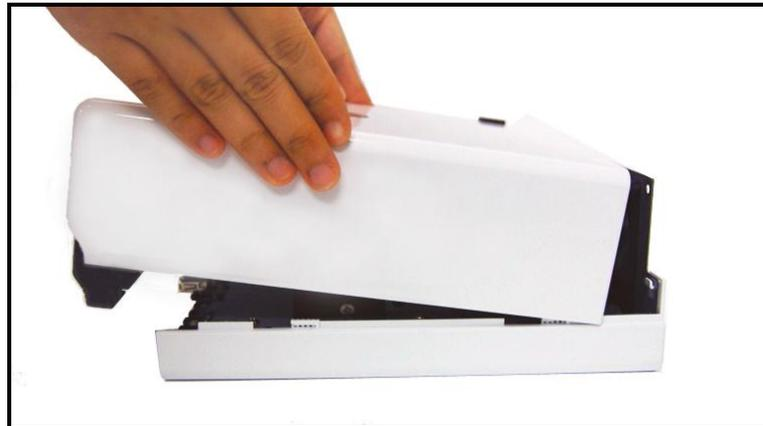
6. Secure the case with the 2 case screws provided.
