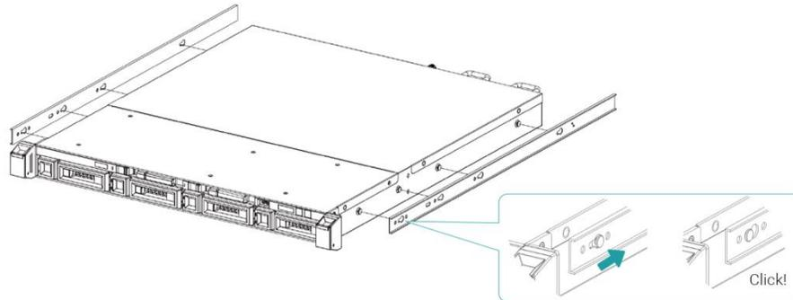
3. Install the outer rail/bracket assembly to the frame. Repeat this step for the other side.
