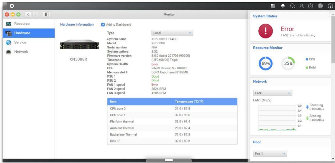
If you see the error message shown above, which means your fan module needed to be replaced immediately. To replace the malfunction fan module, please refer to [chapter 3.4 Replace System Fan](#). After the new fan module is successfully installed, you can see the fan speed displaying its Revolutions Per Minute(RPM) value on QSM.
