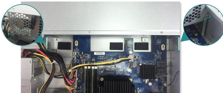
③ Push the fan module all the way down and put the cable back into the cable holder.
