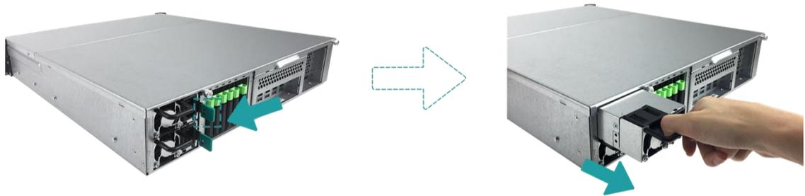
3. Prepare a new PSU, and push it back to the slot until you hear a click. Please make sure that the direction of the PSU is correctly installed, to prevent any potential damage by improper installation.
