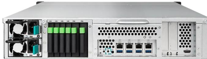
1. Reset network settings: Press and hold the reset button on the rear panel for **3 seconds**, a short beep sound for 1 second will be heard. The administrator password and all the network settings will be reset, the system configuration will result in:
