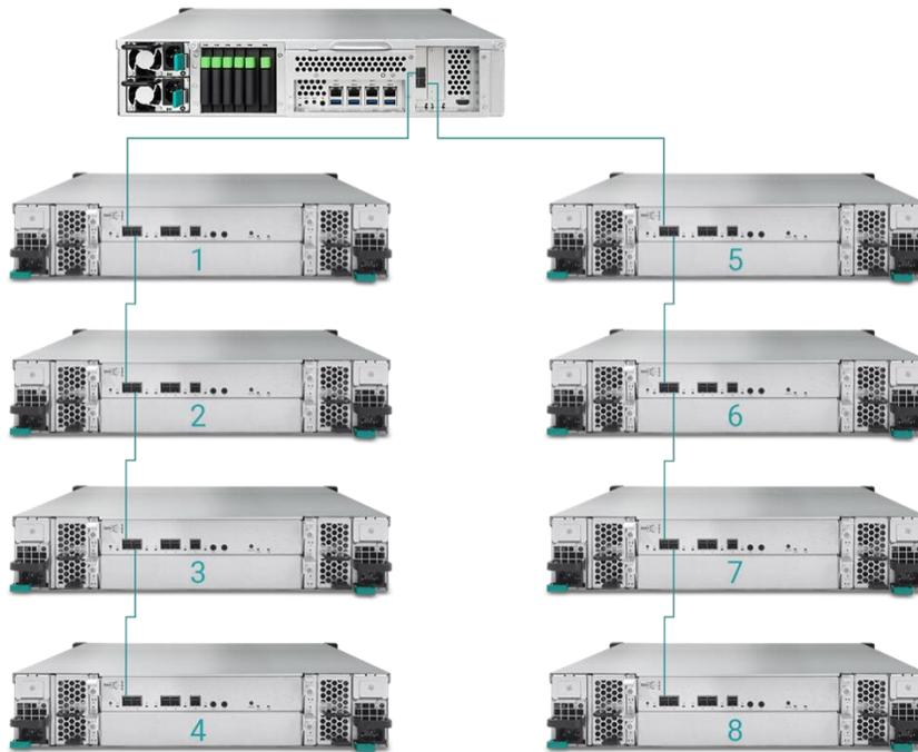
3. After connected to the expansion units, you can check the deployment topology on QSM → Control Panel → Storage app → Overview → Enclosure Map.
