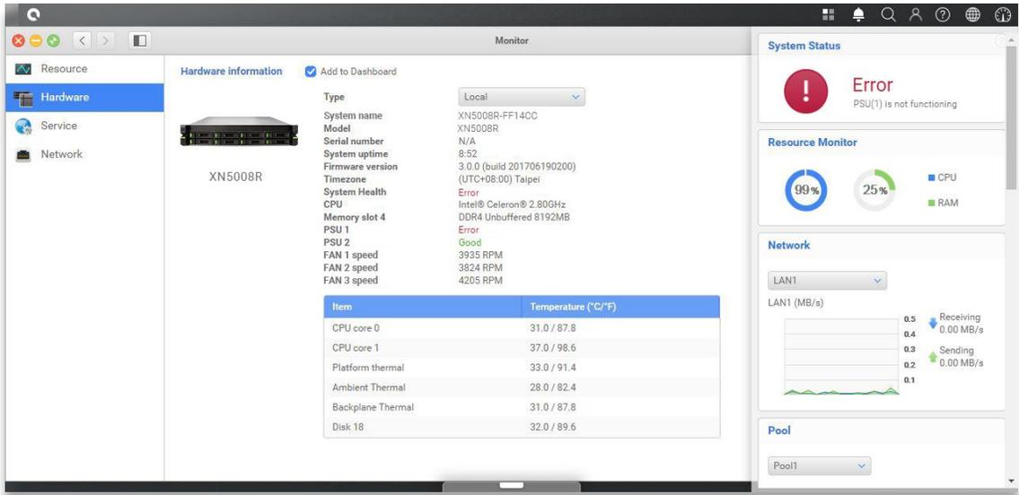
If you see the error message shown above, which means your PSU has encountered an issue and need to be replaced immediately. To replace the malfunction PSU, please refer to [chapter 3.5 Replace Malfunctioning PSU](#). After the new PSU is successfully installed, the PSU status LED will be green and you can see the PSU status displaying “Good” on QSM.
