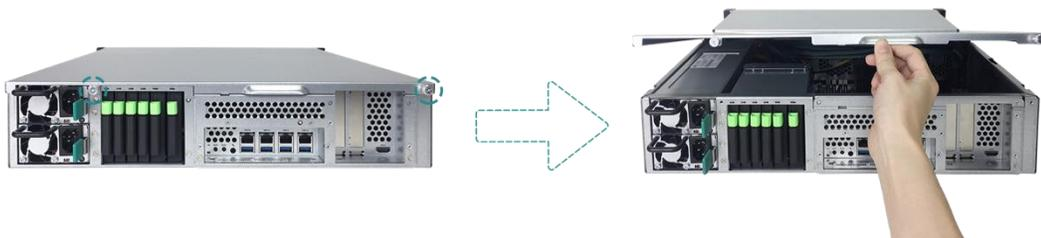
3. Remove the cable on the cable holder and remove the fan module.
