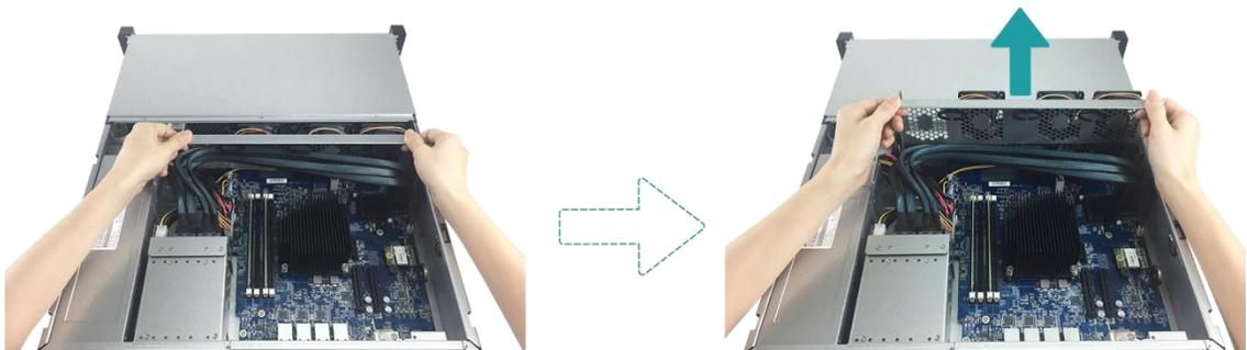
4. Prepare a new fan module and replace the system with the new fan module.
