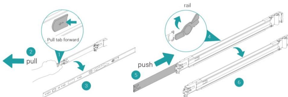
2. Install the inner member onto the chassis.
