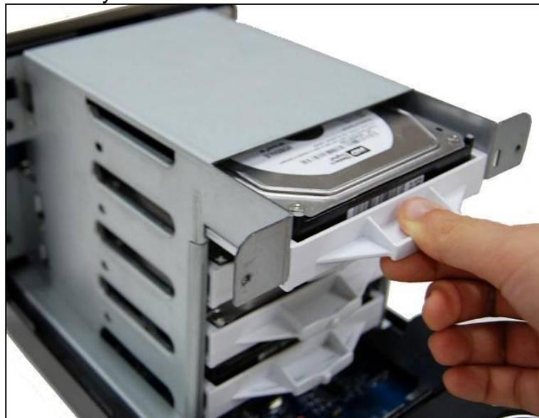
6. If you are using 3.5" hard disks, secure the hard disk trays with the screws (for securing hard disk trays) provided.
