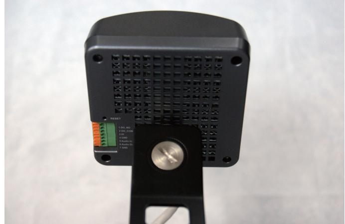
**4. You can adjust the silver screw to fix the angle of camera.**
